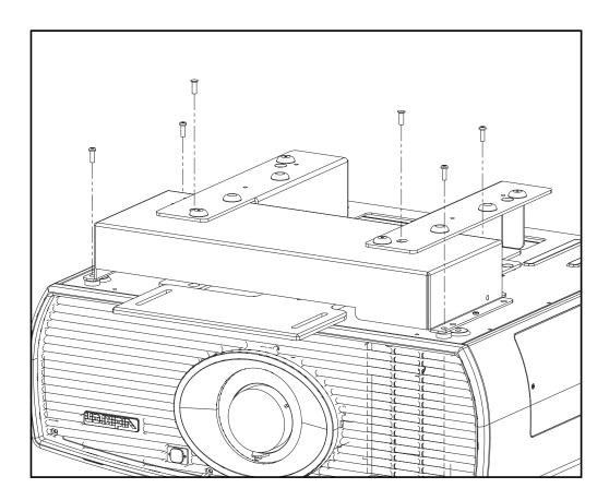
Figure 3-7. AutoScope Lens Motor Installation
